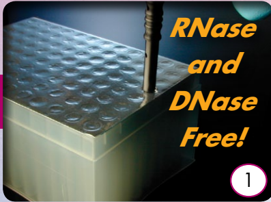
1 Pierce sealing film with handle. Press down and needle or loop will attach itself.
